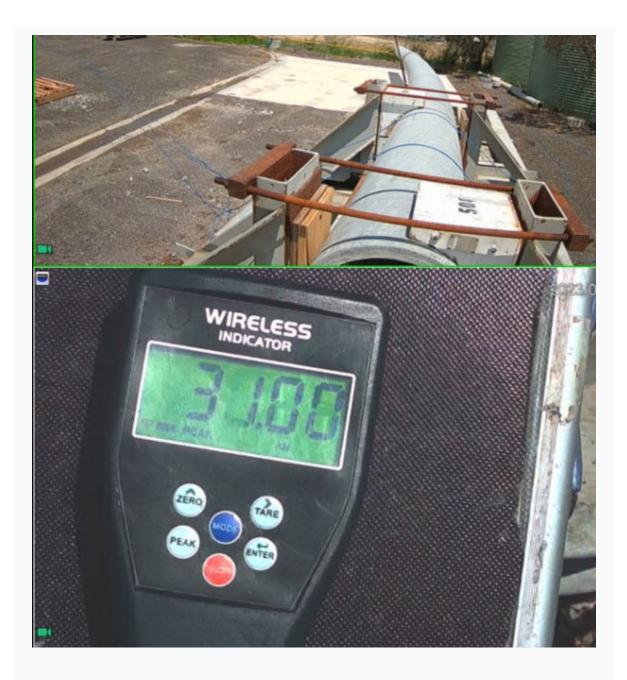
An example above of strength and deviation testing of an engineered 24kN (ultimate) /12.5m Titan prototype sample, which has achieved a breaking load above 31kN.
