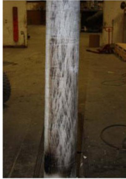
Photos of 7 minutes into the ENA Test with ring burner ignited, as well as radiant heat applied, and the resultant Titan sample showing no distortion of any kind – only shallow cosmetic effect.
