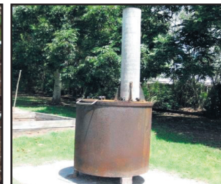
A novel use. Capitalising on the Titan Fire Proof Status, an incinerator chimney made with recycled Titan pole piece.
