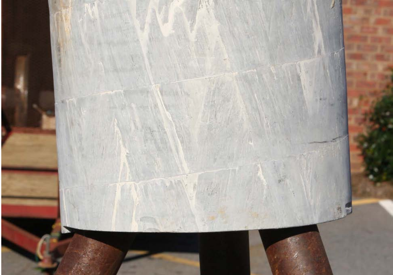
Figure 5. Photograph of tested area directly after the second application of flame
