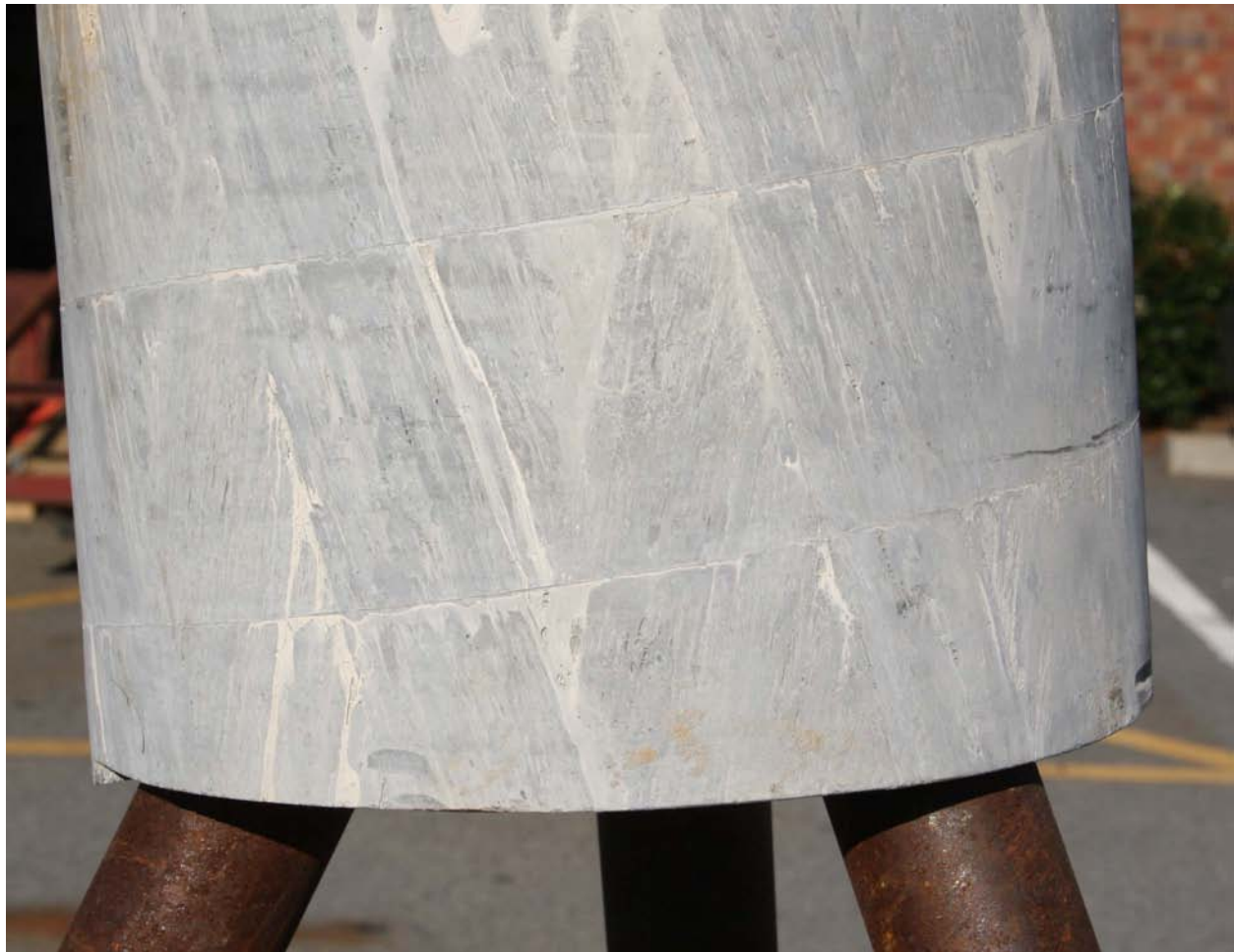
Figure 4. Photograph of tested area directly after the first application of flame
