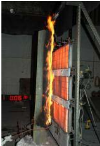
Figure 3. Wood pole specimen six minutes after ENA pole fire test start
